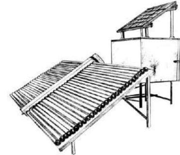
➤ **Solar Powered Cold Storage Unit with Thermal Battery**
